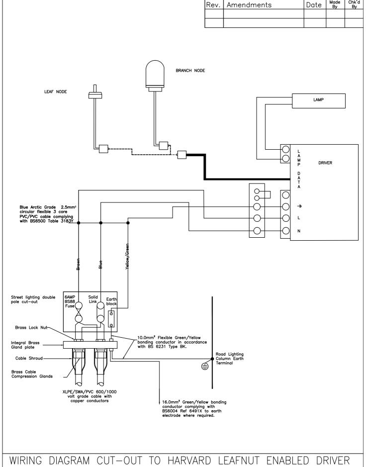
WIRING DIAGRAM CUT-OUT TO HARVARD LEAFNUT ENABLED DRIVER UNIT SUPPLIED BY AUTHORITY XLPE/SWA/PVC UNDERGROUND CABLES
