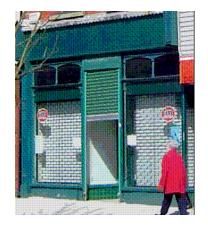
A lattice brick shutter (preferably internal) provides a much more subtle feature than a bulky solid roller shutter.
