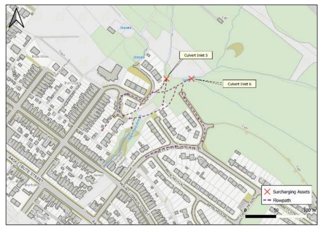
Figure 9: Observed flow paths within 'Treherbert East' sub-catchment during Storm Dennis (16<sup>th</sup> February 2020)
