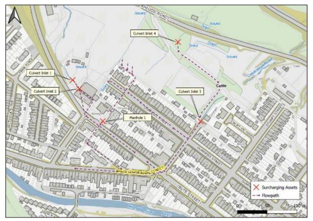
Figure 4: Observed flow paths within 'Treherbert West' sub-catchment during Storm Dennis (16<sup>th</sup> February 2020)
