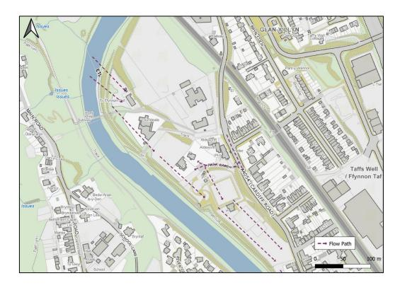
Figure 3: Observed flow paths during Storm Dennis in the north of investigation area RCT17
