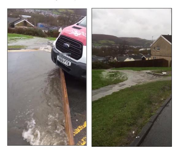
Figure 8: Surface water flows travelling down Maeshyfryd and channelled towards the rear of Tirfounder Road during Storm Dennis (images provided by resident)
