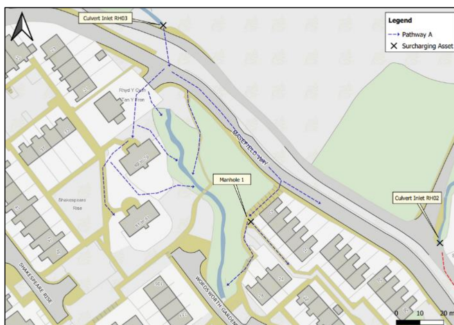
Figure 8: Location of 'Manhole 1' which was identified as surcharging during the storm event
