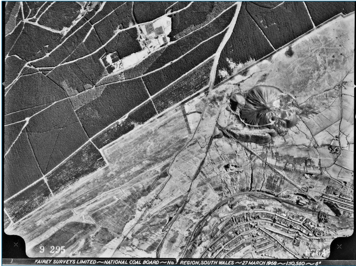
Plate 8. 1968 aerial photograph showing pit features in the vicinity of the proposed Receptor Site suggestive of early mining exploration. © CRAPW
