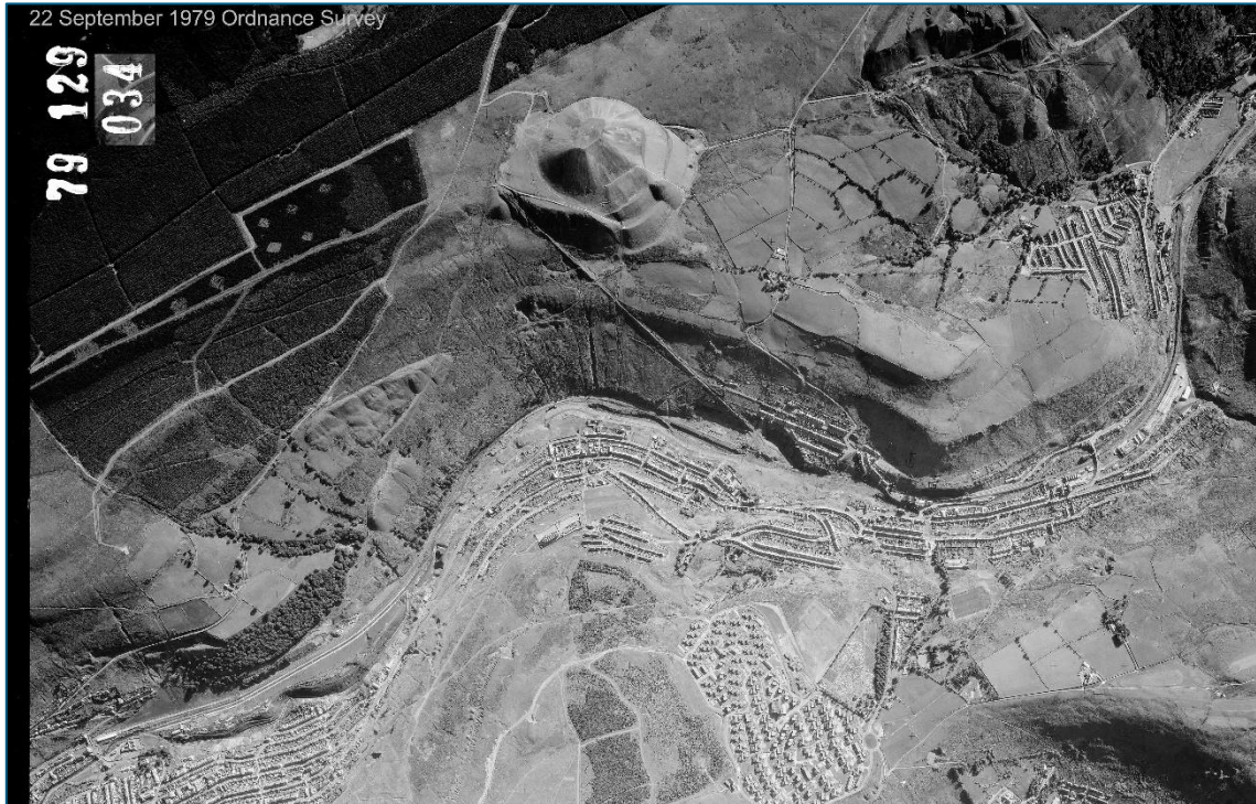
Plate 9. 1979 aerial photograph showing that RH02 'Old Smokey' (TT05) has been landscaped following the closure of the colliery in 1960. © CRAPW
