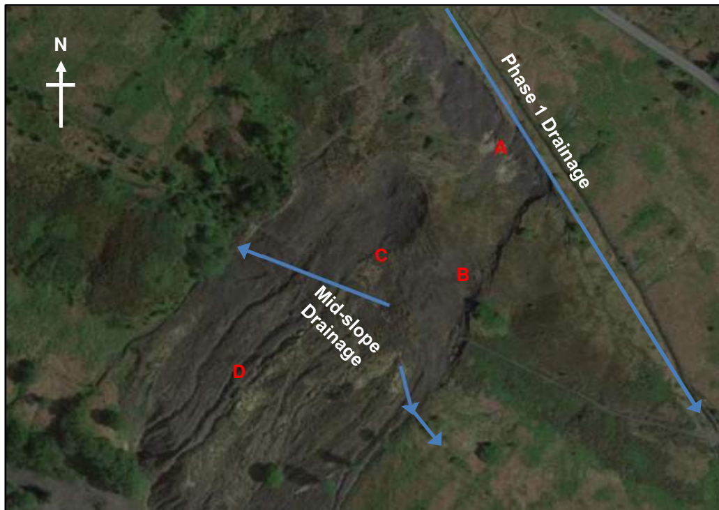
Figure B: Approximate location of on-site observations of water features post landslip
